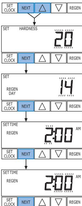
1. Accessed by pressing "NEXT" and ▲ button simultaneously.
